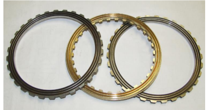
Figure 2 - PolyCone Clutch Pack Assembly
