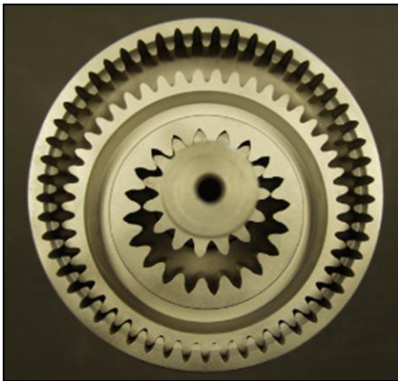
Figure 1 - Addendum Contact Coplanar Gear Arrangement
