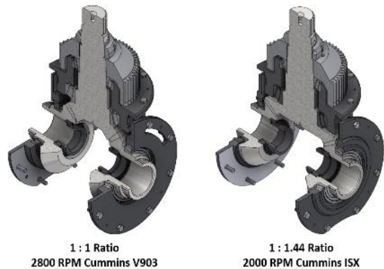
Figure 6 - T-Configuration Input Bevel Variations
